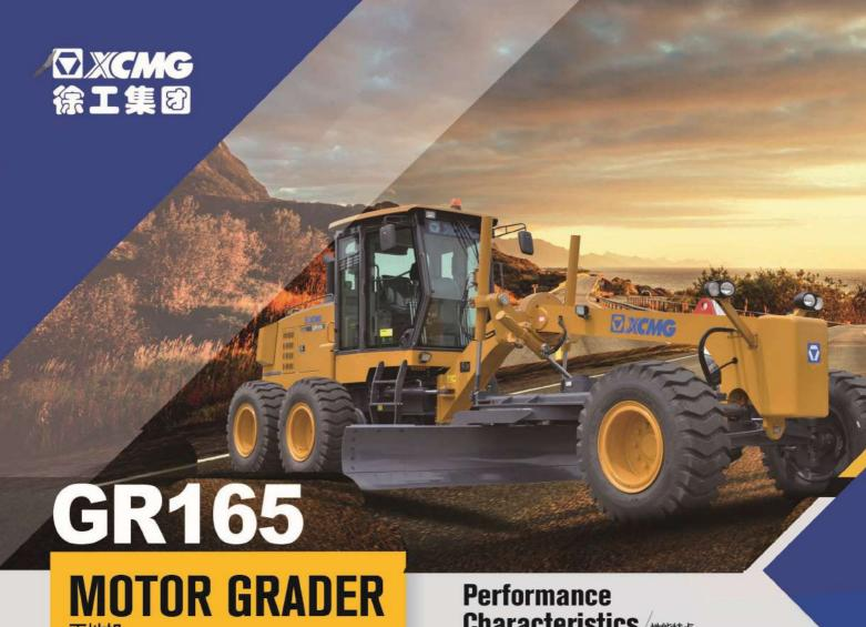
The motor grader is mainly used for ground leveling, ditching, slope scraping, bulldozing, scarification, snow removal for large areas such as highway, airports, farmlands etc. It is the necessary construction machinery for national defense construction, mine con-
